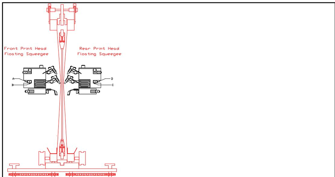
Figure 4 is an example of the front and rear squeegee stroke length set too short. In this example note that both squeegees are extended to the bottom of the squeegee drive bar guide slot at Item B and C, Fig. 4. The front and rear squeegee have both moved to the fixed position. In this instance:
