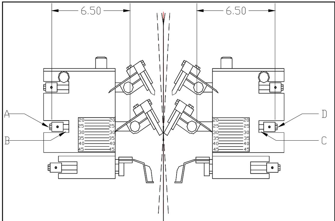
Figure 1, above, indicates approximate squeegee stroke lengths when using a **"Floating/Floating"** squeegee set-up.
