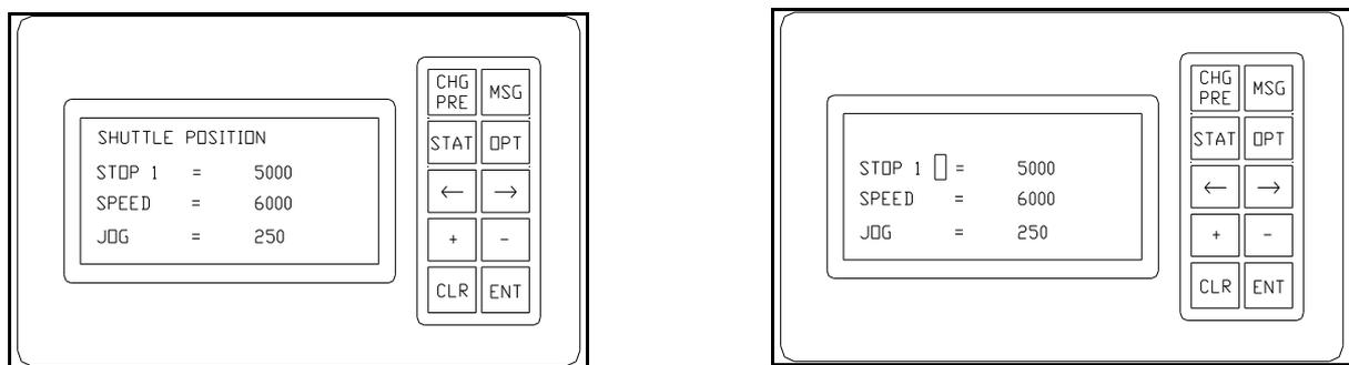
**Figure 7** indicates the Message Screen. No changes can be made from this screen. To access the Edit screen indicated at **Figure 2** Press the **Chg/Pre** button.
