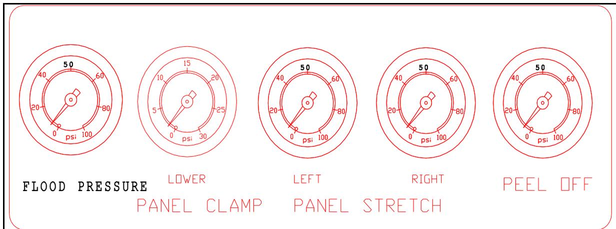
The pneumatic control panel is located at the upper left side of the board load area. Each control consists of a pressure gauge and pressure regulator to monitor and control various functions listed below.
