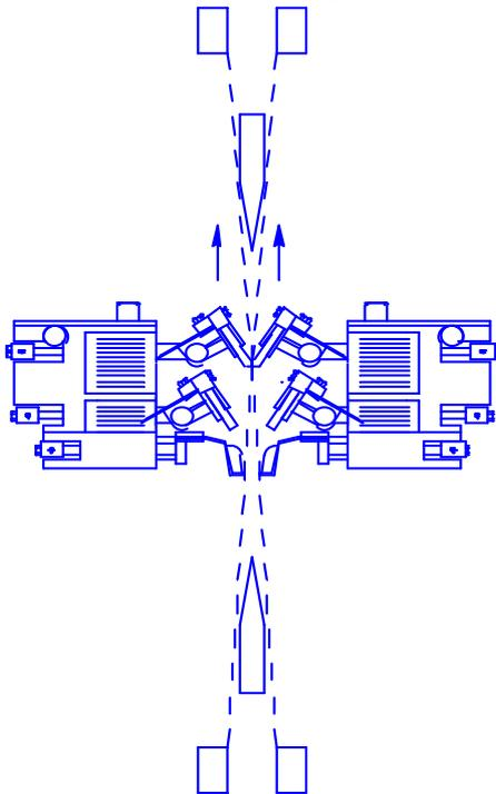
ISOprint System pushing screens together, without a panel in between, to smear the residual LPI ink to the front side of the screen where it is incorporated into the next flood.
