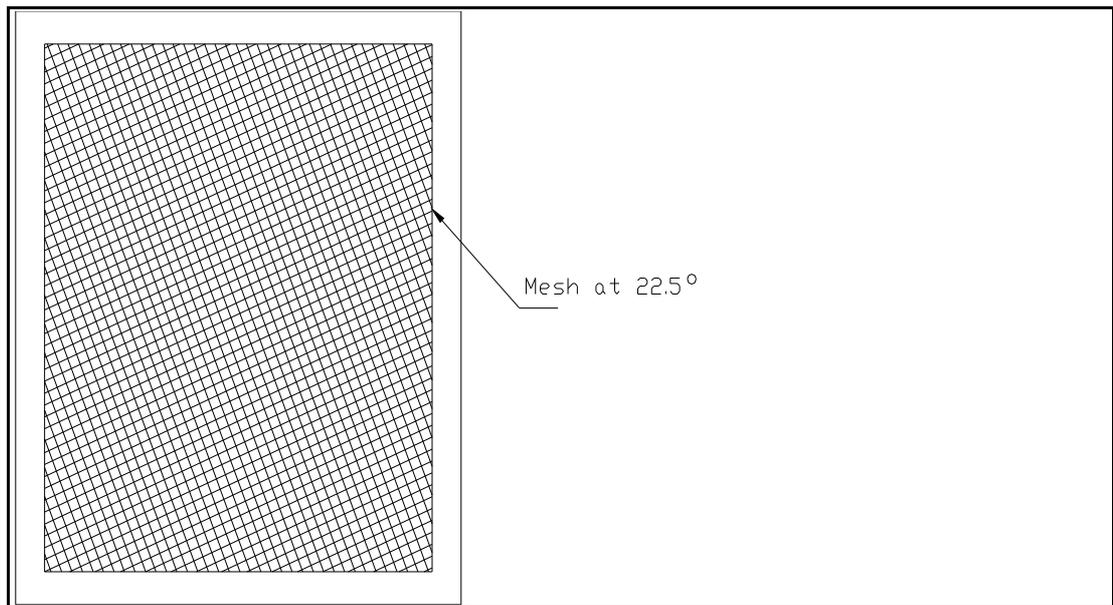
The disadvantages of these types of frames are that they are much heavier than glue type frames. It is difficult to stretch the mesh in them at a perfect 22.5#SYMBOL \f "Symbol"176 angle at the same tension across the frame. The frames tend to bow under higher tensions.
