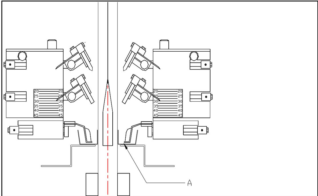
The Flood Bar retract limit is factory set and should not require adjustment. As part of the Flood Bar stroke length check, it is important to verify that the Flood Bar is retracting back far enough that ink will be scooped into the Flood Bar when it extends forward. As indicated in Fig. 6 at Item A, the Flood Bar is positioned with space to move forward and scoop ink into the Flood Bar prior to starting the flood stroke.
