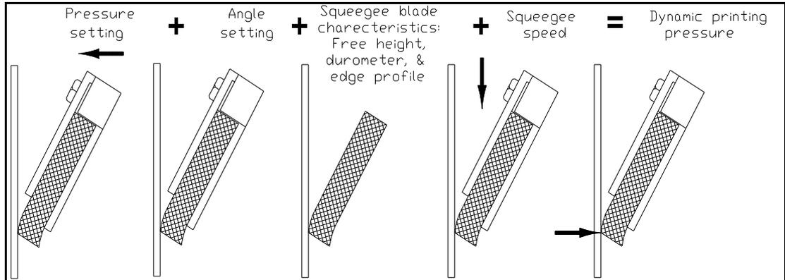
For example, if the dynamic squeegee pressure on the panel is 1 lb/in at 35#SYMBOL \f "Symbol"176 squeegee angle, the pressure on the squeegee may be 60 psi (4.1 bar) at a squeegee speed of 3 in/sec (ips). The same dynamic pressure could also be achieved at 27.5#SYMBOL \f "Symbol"176 angle 100 psi (7.0 bar) at 5 in/sec. All other things being equal, if the dynamic squeegee pressure is the same in two different setups, the soldermask deposit will be also the same.
