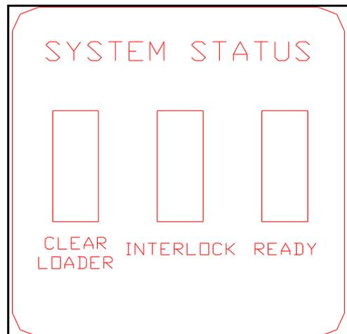
The **CLEAR LOADER** light will be illuminated continuously if a panel does not travel from the load section to the coating chamber.
