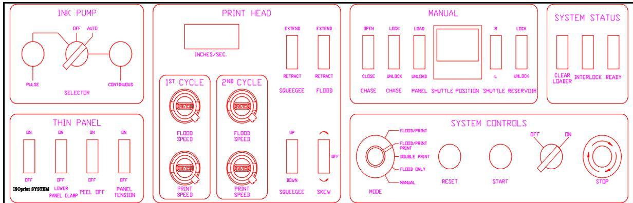
The DP-1500-2X control panel is located on the front of the machine above the coating section. In addition to the control panel, there is an **EMERGENCY STOP** above the coating area doors on the back of the DP-1500-2X, **LIGHT CURTAIN INTERLOCK** in front of the loading section, a **CIRCUIT BREAKER** on the end of the unit below the load/unload area, and a foot switch which functions as a **START** switch.
