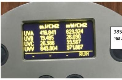
385nm wavelength light energy result at 30% output (2m/min)
