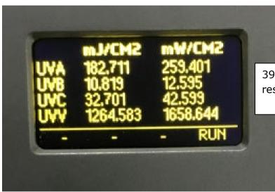
395nm wavelength light energy result at 30% output (2m/min)
