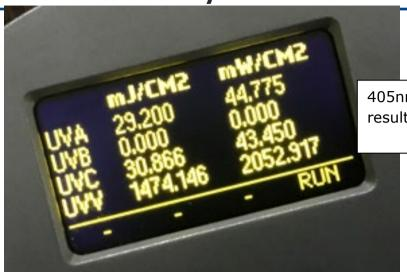
405nm wavelength light energy result at 30% output (2m/min)
