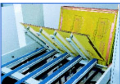
PCB board unloading.
