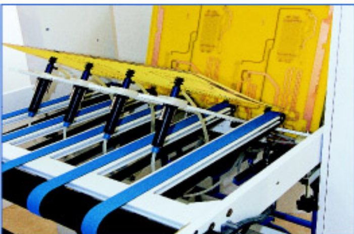
Arms down to place the PCB board on the conveyor.
