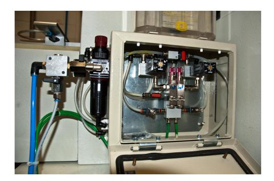
This Kit allows the scoring of Aluminium Boards on a standard machine. It is composed by a cooling device that has to be installed on the standard machine. This cooling device automatically doses and sprays the special coolant on the blades during cutting. It is composed by an external tank which will contains the coolant, a dosing system, all necessary piping inside the machine to carry the mixed coolant to the blades, new designed covers for the blades with copper nozzles.
