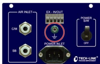
Grounding terminal of electric outlet
