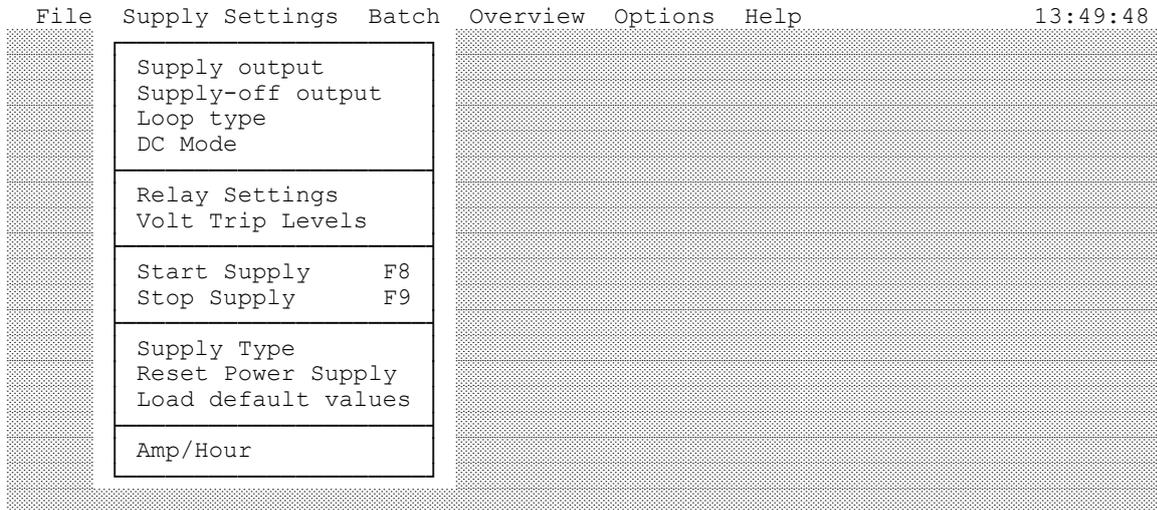
The supply contains a closed loop to control either the output current or the output voltage. To select which output is controlled, use the “Loop type” command. After you’ve selected the loop type, you must set the output currents or voltages and the FwdTime and RevTime. All these parameters can be found in the “Supply Settings menu” with the “Supply output” command.
