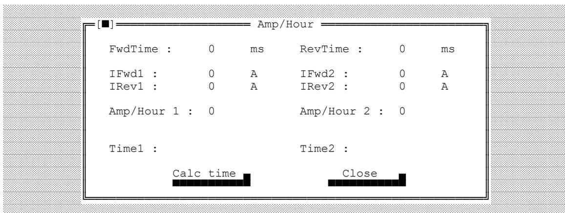
As you can see, the Amp/Hour and time can be calculated for both outputs.
