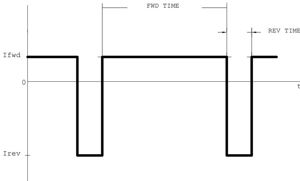
Figure 7.1: The ideal current pattern of a Reverse Pulse Power supply.
