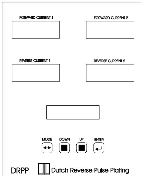
This unit gives access to a menu to control the supply. When the menu is not activated, the LCD-display shows the status of the supply. The keyboard unit is controlled by 4 buttons:
