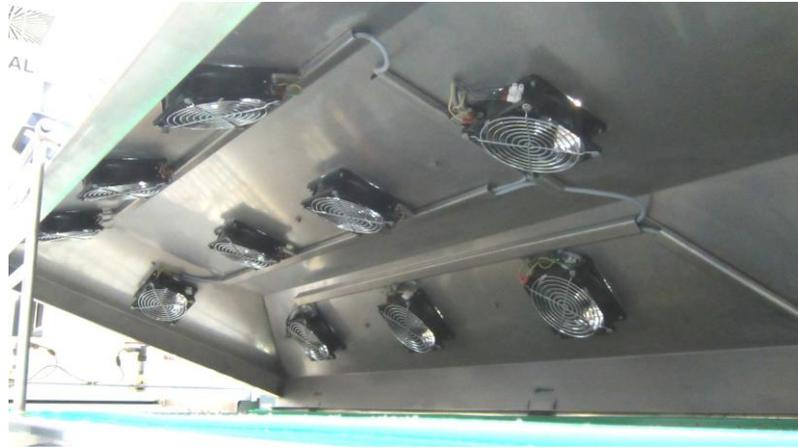
Exhaust: The exhaust is on the cover of the cooling section and must be connected to the exhaust system. The cover of the cooling section is foldable, thus the connection of dust extraction must be done via a flexible hose or a pipe which is cut at an angle of 45°. The exhaust port is 100mm in diameter and requires a throughput of suction capacity of 300m<sup>3</sup> / h.
