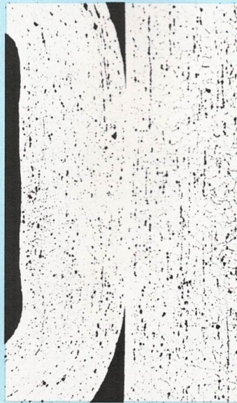
Molybdenum Honeycomb Mag.: 50X Etchant: As Polished
