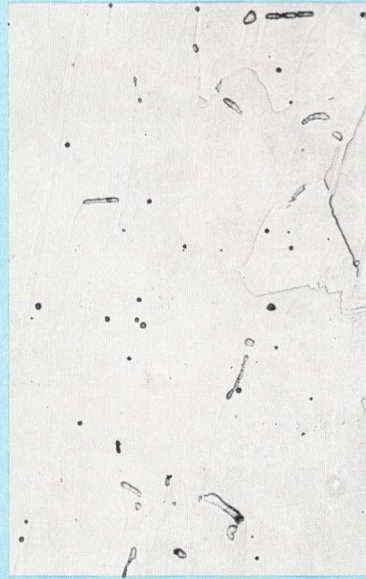
Silicon Substrate Mag.: 100X Etchant: Attack Polished
