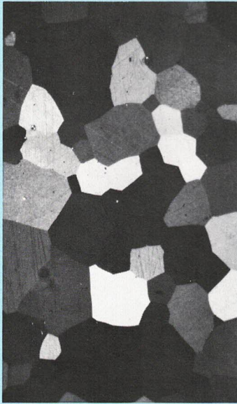
Beryllium Alloy Mag.: 50X Etchant: As Polished (Polarized Light)
