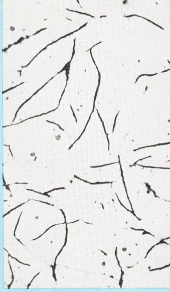
Gray Cast Iron Mag.: 100X Etchant: As Polished
