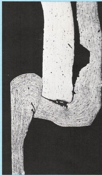
Aluminum Can Top Upset Weld Mag.: 50X Etchant: Kellers
