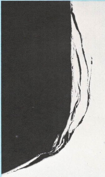
Steel Screw with Thread Defect Mag.: 100X Etchant: As Polished
