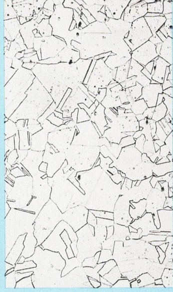
50 Nickel-50 Iron Mag.: 100X Etchant: Nitric Acid (HNO 3 ) Acetic Acid (CH 3 COOH)
