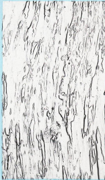
Tungsten Mag.: 50X Etchant: As Polished
