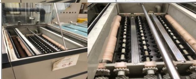
NEUTRALIZER MODULE LENGTH 670mm
