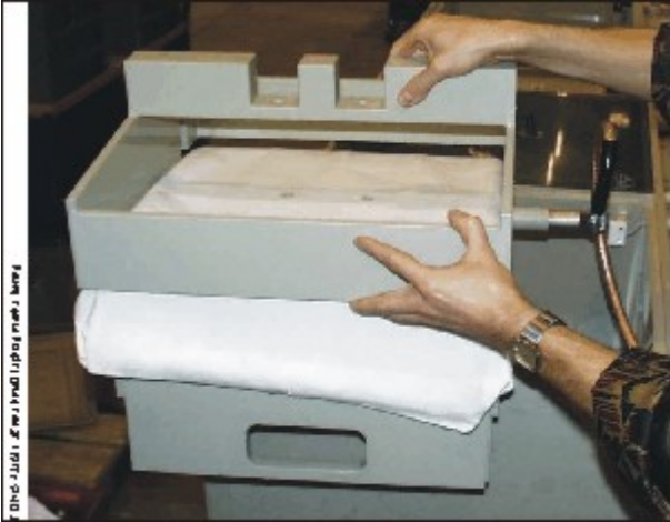
Removing holding frame for diaphragm
