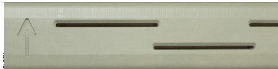
SFD: Slots with chamfer at front side; Arrow, to mark the direction of transport
