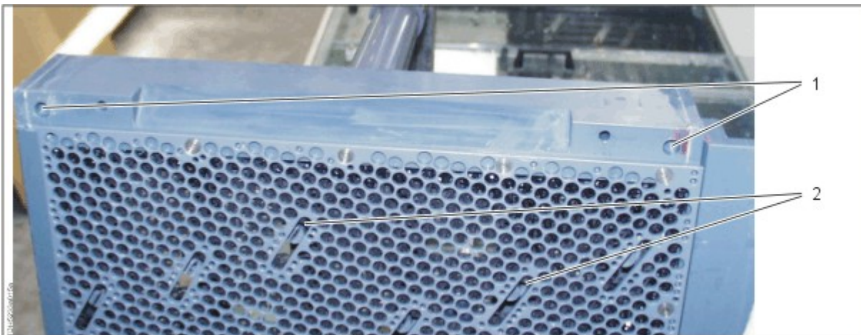
Upper anode segment removed and lifted
