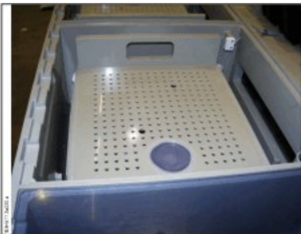
Anode box in the Redumat compartment
