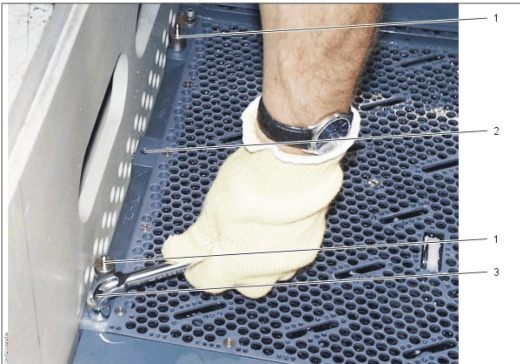
Nuts for fixing the bottom anodes with 13 mm spanner
