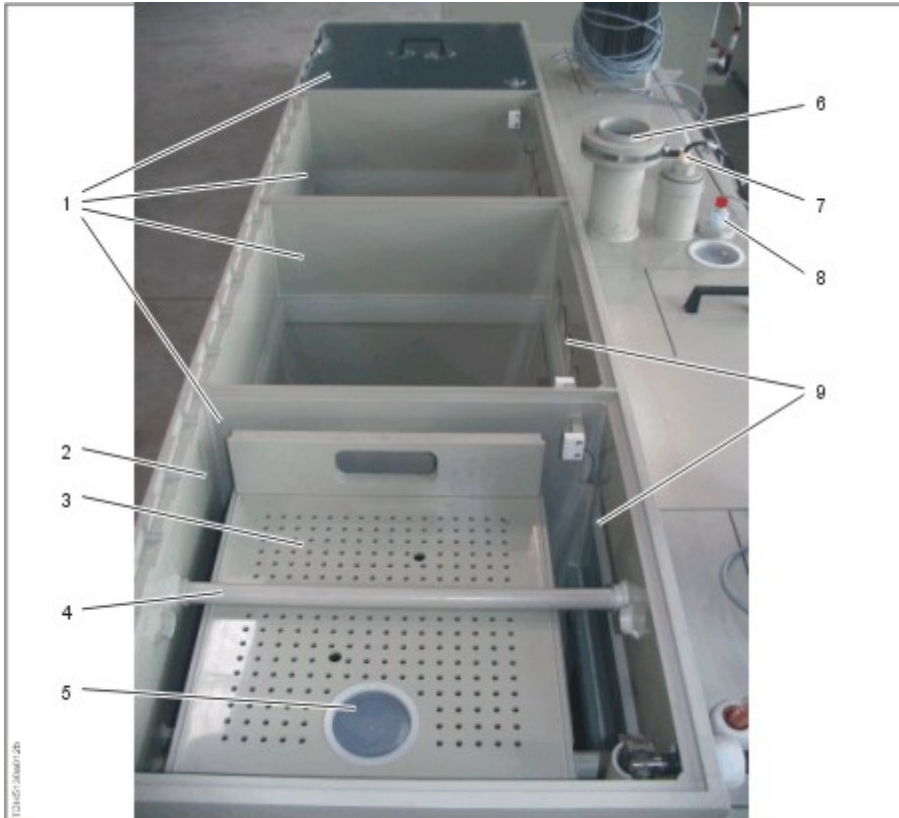
Top view of Redumat compartment and three Copper Dissolving compartments
