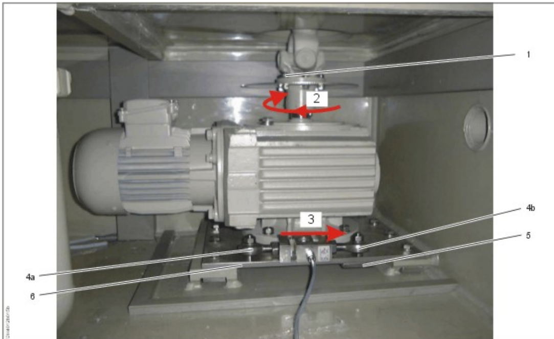
Clamp drive motor with tensile force sensor
