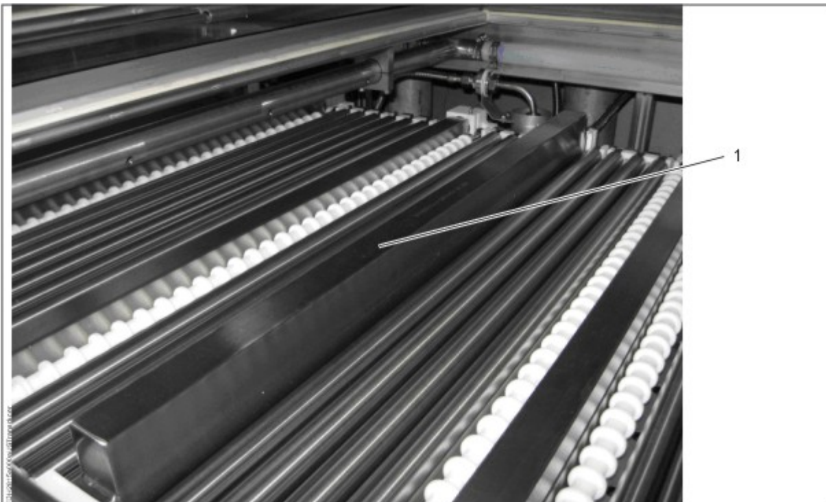
[1] Ultrasonic transducer integrated in conveyor of module (line not operating!)
