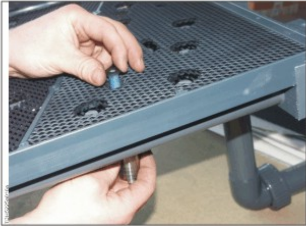
Mounting of distance bolts
