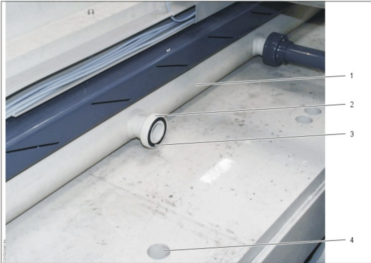
Mind the O-ring, when removing or remounting the anode unit
