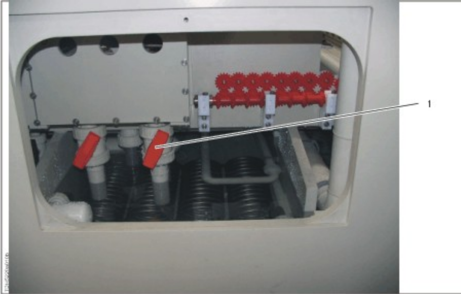
Manual valve for the adjustment of fluid return flow during line commissioning
