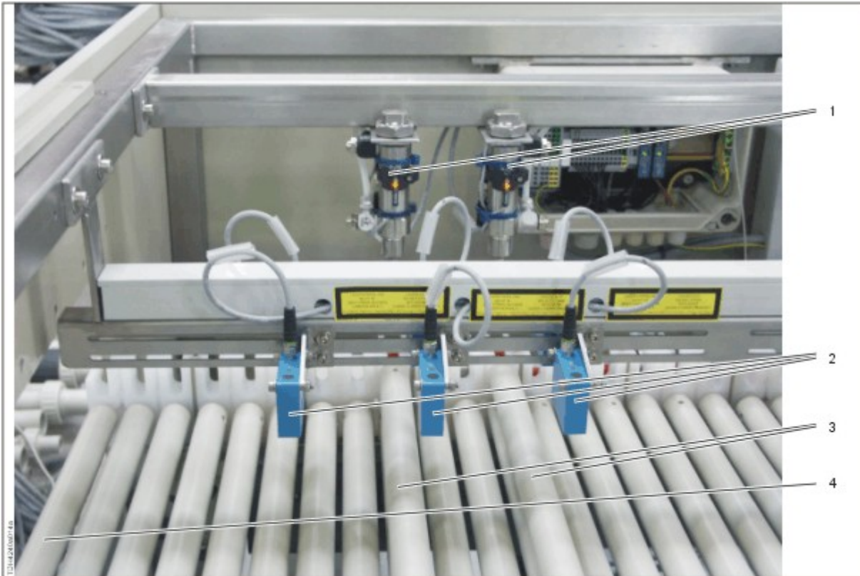
Gap adjustment in outlet section of the CGA
