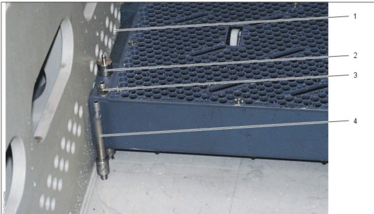
Base bolts on which the anode units are resting (for height adjustment)
