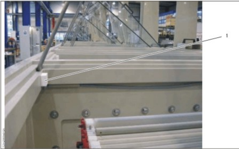
Cover switch actuates an alarm when the magnetical effect is interrupted
