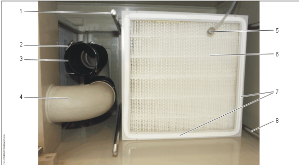
View into the opened bottom compartment of the Dryer module (here with the holding frame of the HEPA filter already removed)
