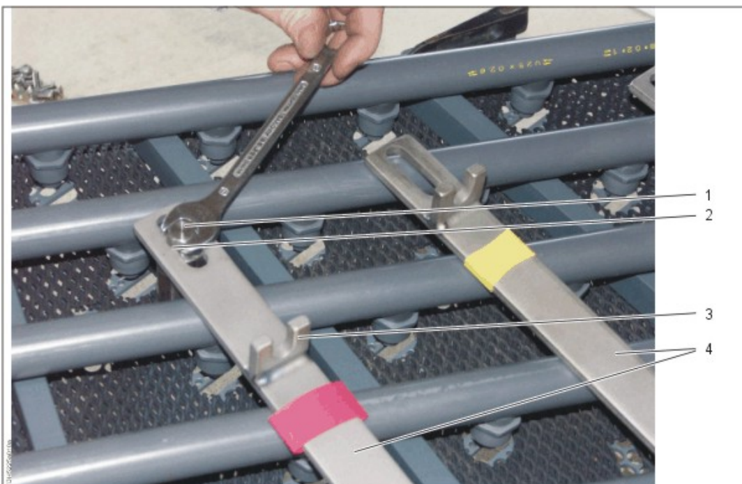
Removal of connection bars
